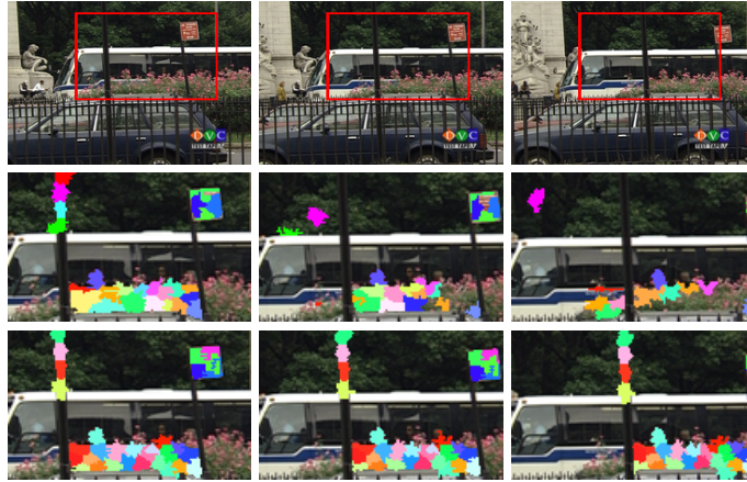
Fig. 6. Example for a challenging segmentation task with low contrast and high motion. Top row shows the original sequence with a marked area magnified in the rows below. For the two lower rows a full segmentation was performed with the baseline approach (BL, middle) and the proposed approach (BL+BP+CE+MM, bottom). Only a subset of superpixels is shown, which was manually selected and colored. Same color means temporal connectedness. In the middle row the superpixels are torn away by the motion introduced by the camera panning, while they keep their position and constellation for the proposed approach.
